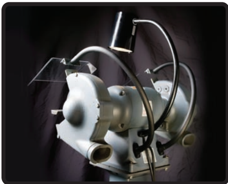
Rear view of the above pedestal grinder showing the direct-mount bases of the shield assemblies.
