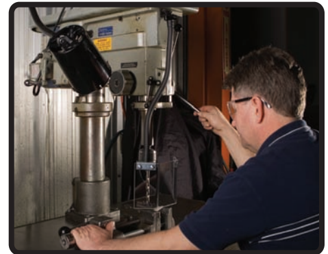
SHD-18106W shield assembly mounted on a drill press with a BKT-150 horizontal right-angle mounting bracket.
