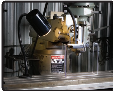
SHD-12169U shield assembly mounted on a milling machine with a BKT-150 horizontal right-angle mounting bracket.
