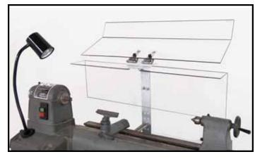
Shield in the up position for changing the workpiece. Be sure to move the shield back into the down position before operating the lathe.
