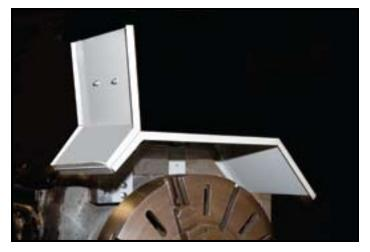
The front portion of the lathe shield can be hinged up for easy access to the chuck or workpiece. When turning a workpiece while the front portion is hinged up, additional safeguarding must be used to protect individuals.
