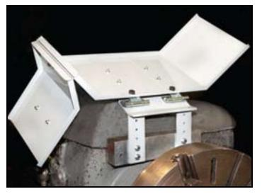
Shield in the up position for changing the chuck or workpiece. Be sure to move the shield back into the down position before operating the lathe.
