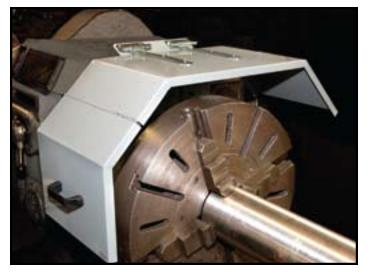
Shield in the down position when operating the lathe. When installing the shield, make sure it clears all parts of the chuck.
